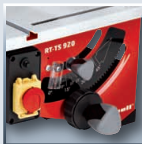
Saw blade adjustment (height and angle)
