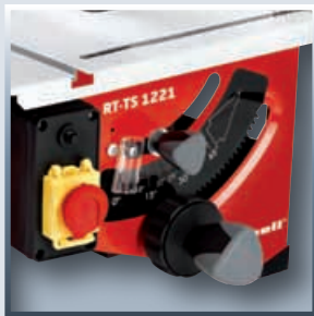
Saw blade adjustment (height and angle)
