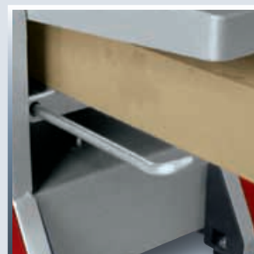
Thickness planer with pull-out workpiece support
