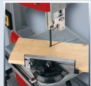
Infinitely variable angle stop
