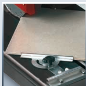
Precisely adjustable stop
